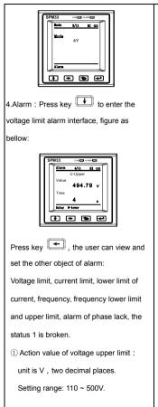
Notice: action value of voltage upper limit must be greater than voltage lower limit. Can be set to"0","0"indicates that the alarm type is closed.
