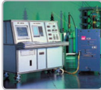
Characteristics Test / VCB Characteristics Test
